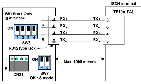
Figure 3.2.1.1b S Mode(Basic BRI Line Connector and Terminating Resistors)
